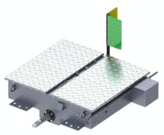
The YM-16 is an electric over hydraulic switch machine with a unique patented actuation and holding force design for a smooth operation with any size switch point. It's designed to be a direct replacement for hand throw or power switch for any yard. For added safety the machine can be trailed through at up to 30 mph without any damage.
